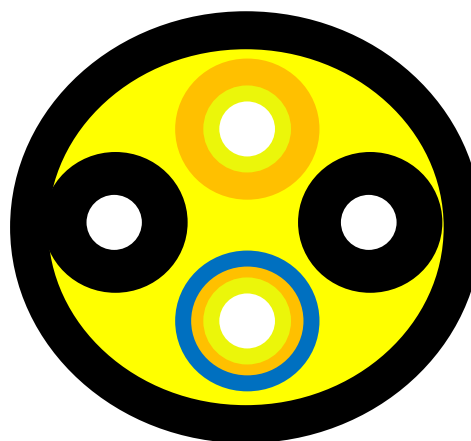
7.0mm LSZH Jacket with Two 2.0mm SM or MM Fibers & Two Stuffing Cable
